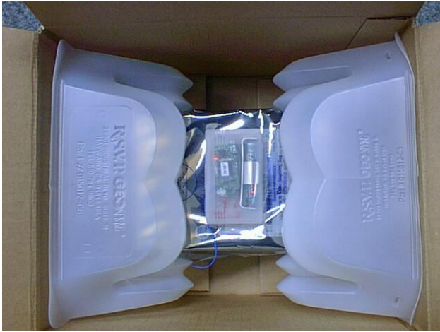
A hard disc drive with an eSeal based on particle computer
